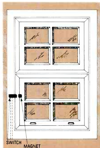
FIG. 5—A MAGNETIC REED SWITCH can also be used to make sure a window is closed. When the magnet is next to the reed switch, the switch closes. When the window is opened, the switch opens.
